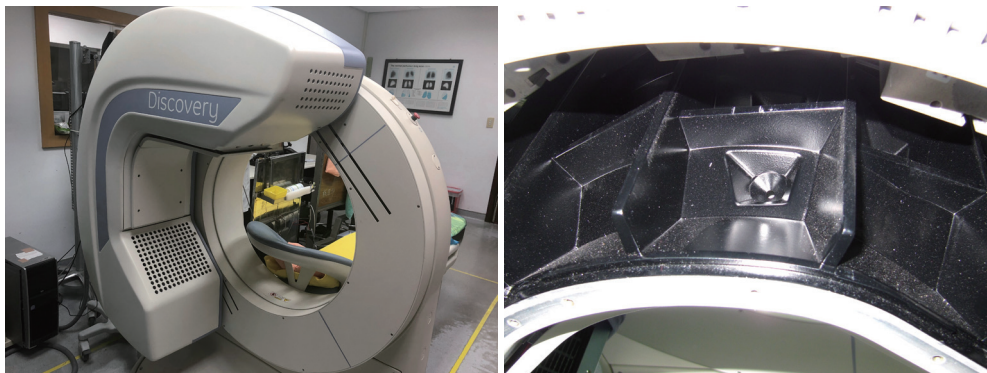
Figure 12 Left: Discovery NM 530c featuring a gantry that is similar to a conventional cardiac SPECT camera, with a different detector assembly that allows completely stationary acquisition. Right: sample pinhole aperture from Discovery NM 530c (courtesy of Taipei General Veterans Hospital).
