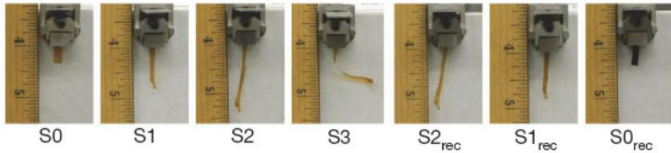
Fig. 5. Quadruple-shape memory properties of PFSA. S0: permanent shape; S1: first temporary shape ( $T_d^1$ : 140 °C); S2: second temporary shape ( $T_d^2$ : 107 °C); S3: third temporary shape ( $T_d^3$ : 68°C); S2<sub>rec</sub>: recovered second temporary shape ( $T_r^1$ : 68°C); S1<sub>rec</sub>: recovered first temporary shape ( $T_r^2$ : 107 °C); S0<sub>rec</sub>: recovered permanent shape ( $T_r^3$ : 140 °C). (Adapted with permission from (Xie, 2010). 2010. Nature Publishing Group Inc.)
