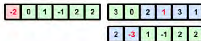
Figure 4.5: Each iteration of the genetic algorithm goes through a set of recombination, mutation, and selection in order to form the next generation. Here we use the generation initialized from Figure 4.4 as an example of how recombination, mutation, and selection would work to generate the next set of solutions.
